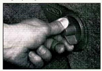
Remove your jack cover by turning the plastic wing nut counterclockwise.
